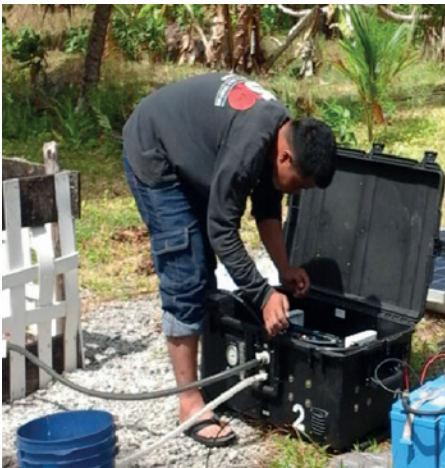
Reverse Osmosis (RO) Machines in the Marshall Islands: A 360 gallon per day RO unit on Namu Atoll. Source: IOM - Situation Report #2 Marshall Islands
